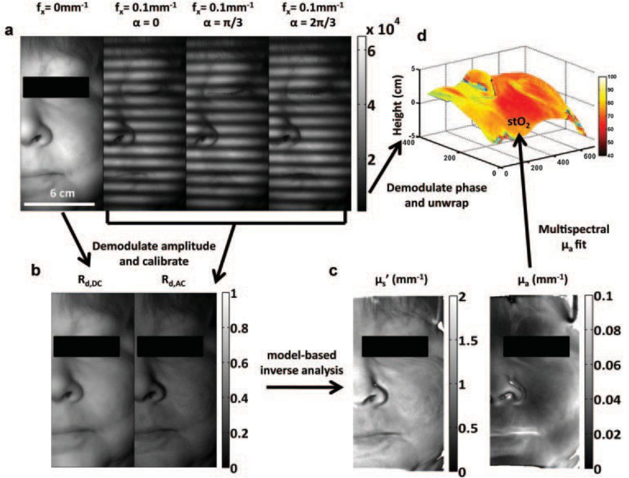
Fig. 1. Data flow in SFDI. **a**: Patterns are projected onto tissue sample and then **(b)** demodulated and calibrated to a known standard. **c**: A pre-calculated look-up table is then used to derive tissue optical properties on a pixel by pixel basis.
