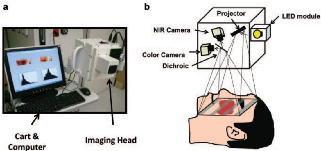
Fig. 2. **a**: A compact and lightweight LED-based instrument used for the clinical measurements described herein. **b**: A typical SFDI system consists of three fundamental components: a light source, a spatial light modulator, and a camera.
